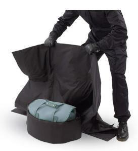
Used by law enforcement, military, and close protection teams VestGuard hard or soft armour ballistic containment rings can be quickly deployed around IEDs, unsafe weaponry, ammunition, and other possible explosive devices to contain the threat, and capture the blast including any projectile fragments. Designed to work in-conjunction with a ballistic blanket cover to fully control the threat. Manufactured to order and designed to meet each individual requirement.
